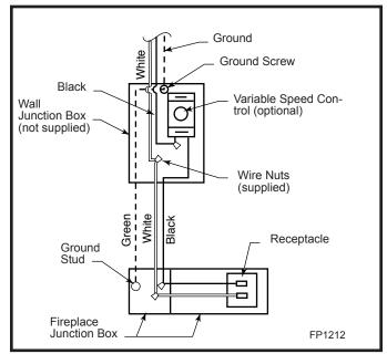
Fig. 9 SCVS wiring diagram.
